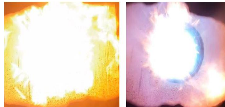
Figure 7 Comparison of the appearance of the petroleum No. 2 fuel flame (left) and the EL flame (right). Both at ~6.5% flue gas oxygen and a nominal input rate of 1.4 million Btu/hr.
